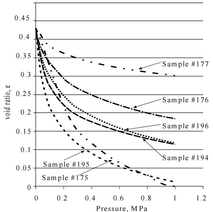
Figure 2. Compression curves for argillite samples (with full water saturation)
