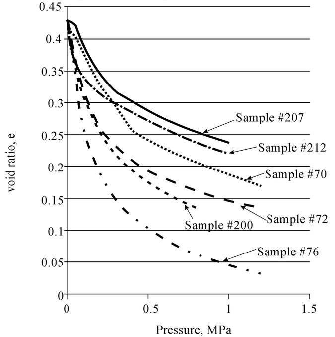
Figure 1. Compression curves for argillite samples (without water saturation)
