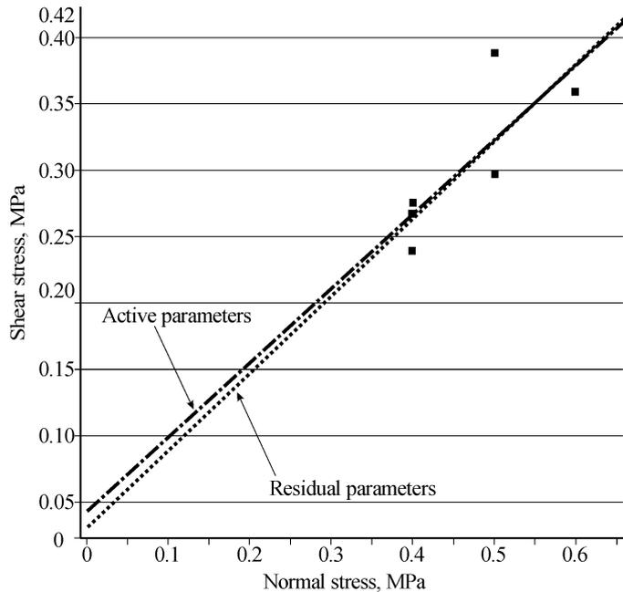
Figure 3. Argillite samples strength straight lines
